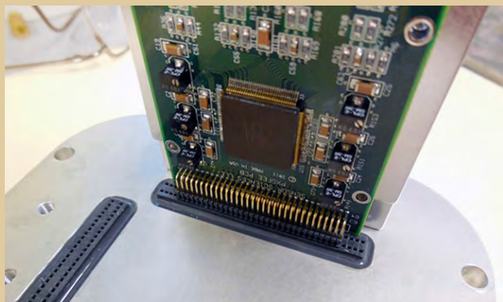
Fig. 8. External side of detector showing 80 contact feedthroughs ( \times 2 ) sealed with epoxy and a 64-channel preamp board plugged into one axis.
