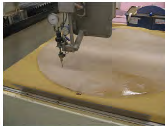
Rounding the glass face plate
