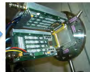
Two small, low-mass, low-power ASIC and FPGA boards qualified for flight
