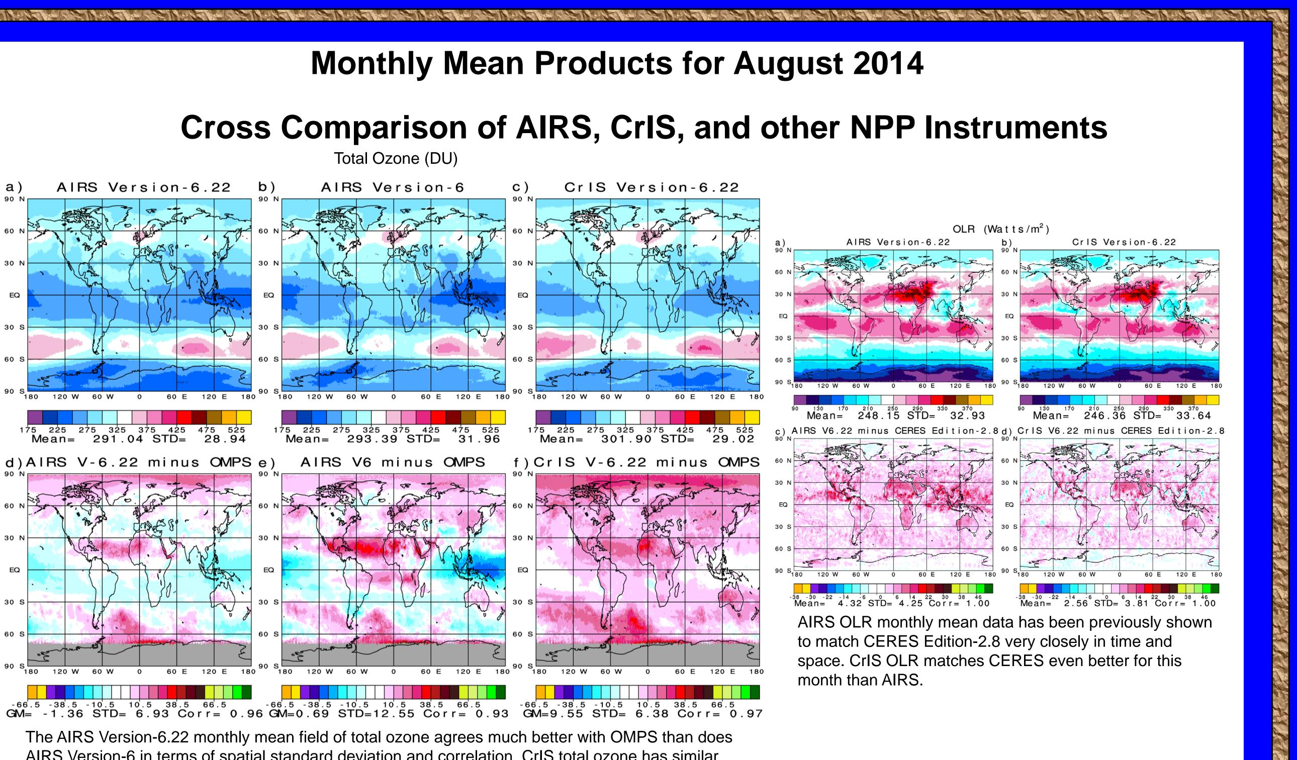
AIRS Version-6 in terms of spatial standard deviation and correlation. CrIS total ozone has similar standard deviation and correlation with OMPS as AIRS, but is biased high. We are continuing to improve details of the ozone retrieval algorithm and QC procedures.
