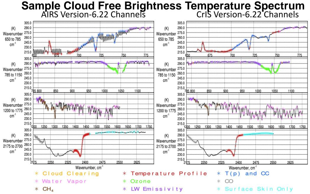
Sample AIRS and CrIS brightness temperatures computed for a cloud free scene. The AIRS and CrIS channels we use in different steps in the retrieval process are indicated in the figures by different colored stars. AIRS is sampled twice as densely as CrIS and extends further at the high frequency
