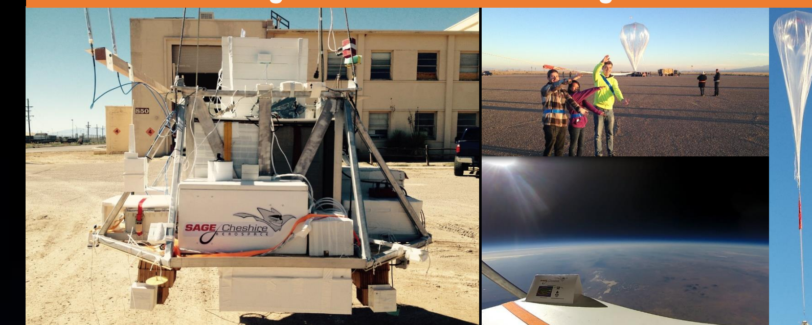
Fig. 9 Sage Cheshire high altitude balloon launch. Successful operation of OPTI in near space environment (no laser or time transfer test was performed).
