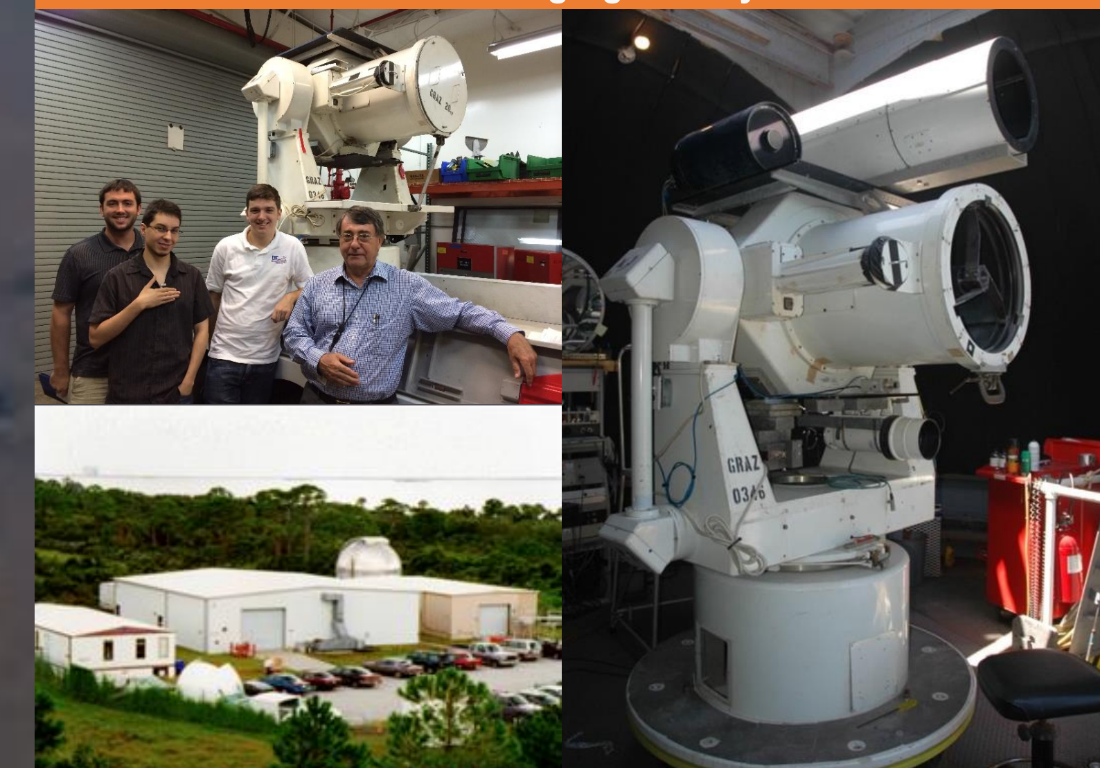
Fig. 11 Satellite Laser Ranging (SLR) facility operated by Townes Institute Science & Technology Experimentation Facility (TISTEF) managed by University of Central Florida at Kennedy Space Center. Collaboration includes a 1064 nm laser with 50 cm satellite tracking telescope and 1 km test range. [3]
