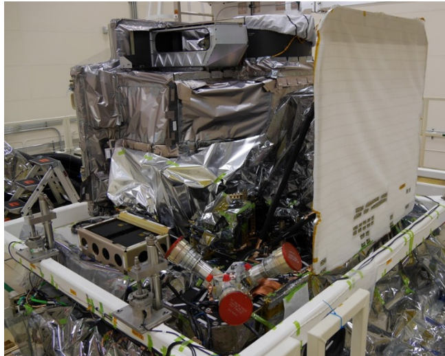
Figure 4. GOES-R EPP populated with instruments and AD sensors.
