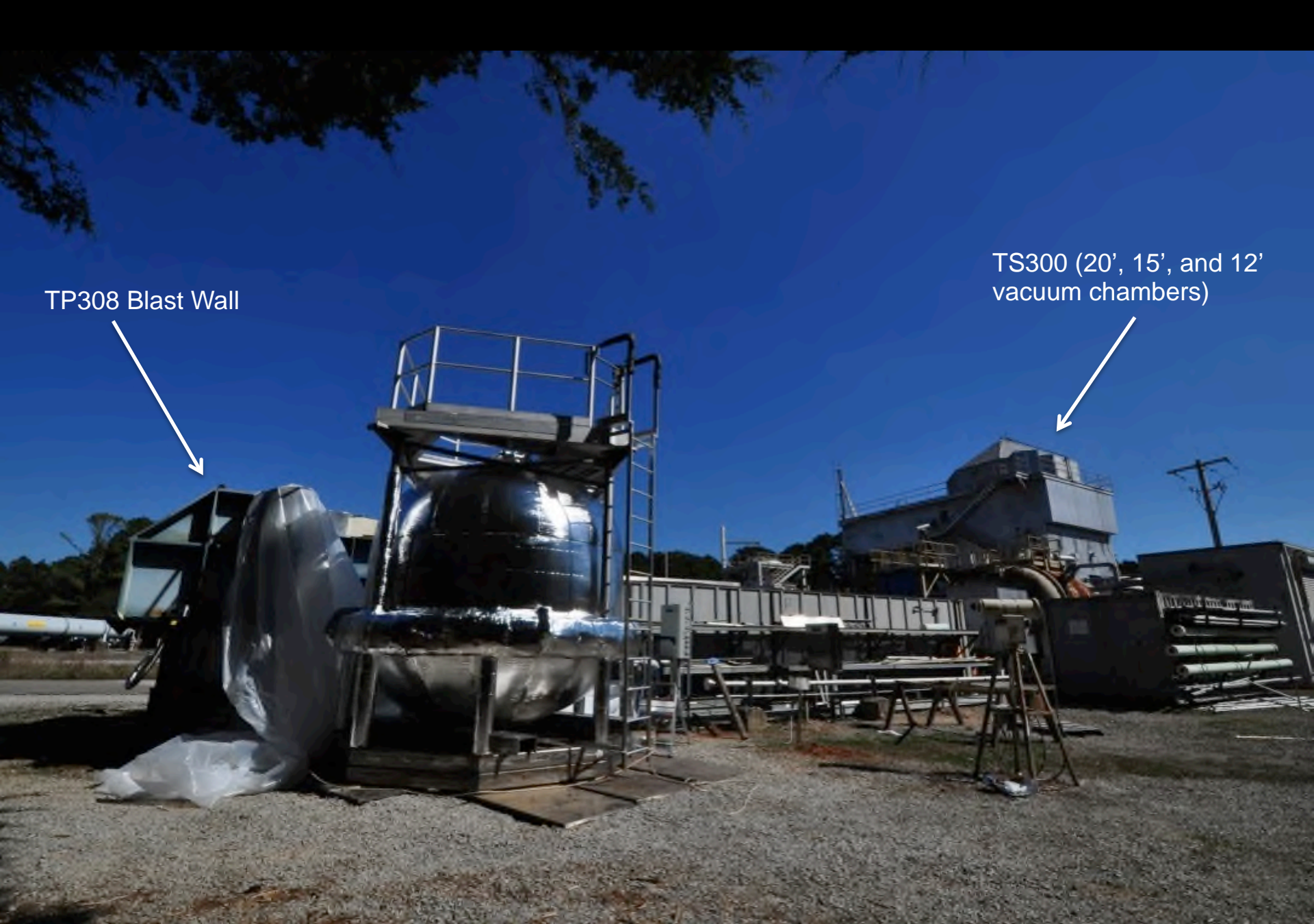
CRYOTE3 placement at TP308 in the MSFC East Test Area
