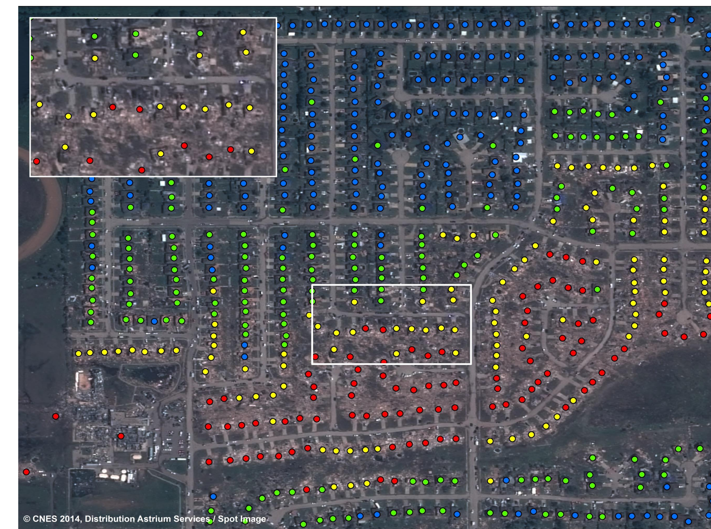
Figure 3. Example of experimented methodology exploring what damage can be seen from high resolution imagery
