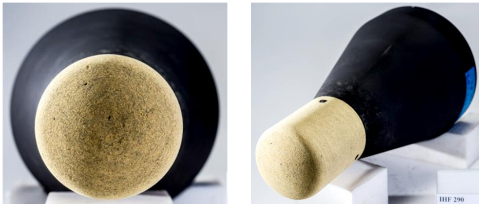
Figure 11: Top view and side view of PICA samples prior to arcjet test.
