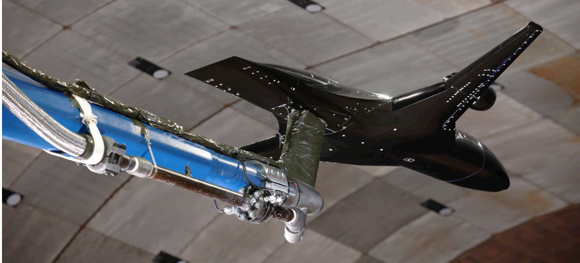
Figure 4.15. AMELIA installed in the tunnel with empennage removed.
