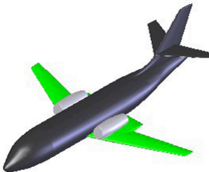
Figure 2.2. Configuration 2 is comprised of a high aspect ratio wing, over the wing engines, circulation control at the trailing edge and a cruciform tail.
