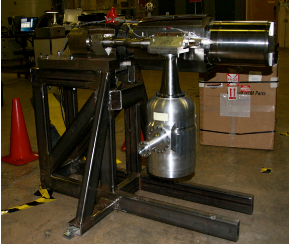
Figure A5.5. Zero thrust body mounted to right side slot blowing plenum of balance assembly.
