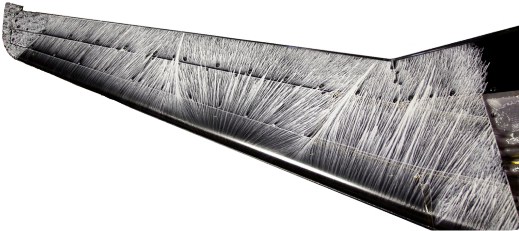
Figure 10.16. Slot Flow Calibration Oil Flow Visualization: 12% Dense Metal Foam.
