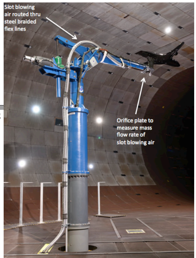
Figure 5.3. Photo showing model support system and slot blowing air routing.
