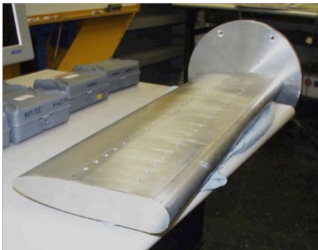
Figure 10.1. Elliptical circulation control airfoil model with rounded trailing edge.
