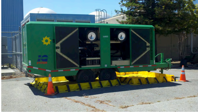
Figure 10.11. Air compressor used for the slot flow calibration effort.
