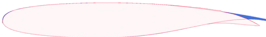
Figure 4.11. AMELIA's modified airfoil (pink) over the original NASA SC(2)-0414.
