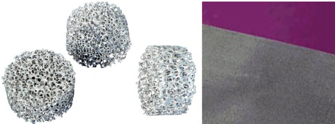
Figure 10.10. Samples of metal foam and woven metal mesh used in the circulation control plenums (images courtesy of ERG Aerospace and the Pall Corporation).
