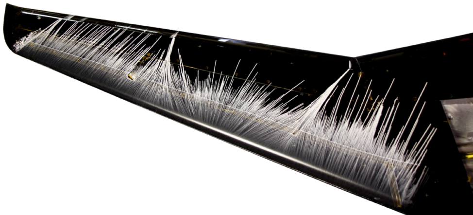
Figure 10.15. Slot Flow Calibration Oil Flow Visualization: 6% Dense Metal Foam.
