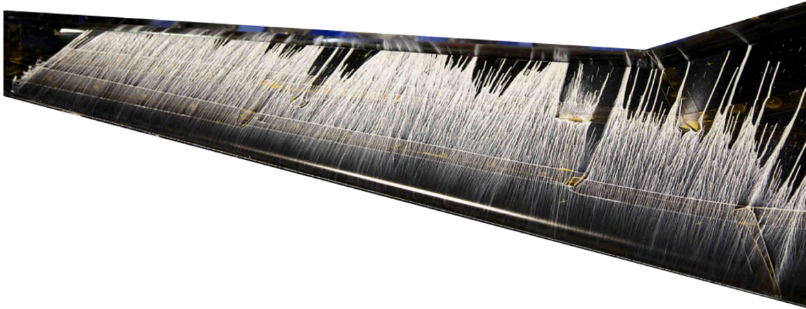
Figure 10.19. Slot Flow Calibration Oil Flow Visualization: 12% Dense Metal Foam + Rigimesh.
