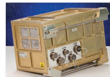
The LMM control box contains the control avionics for the entire LMM subrack facility.
