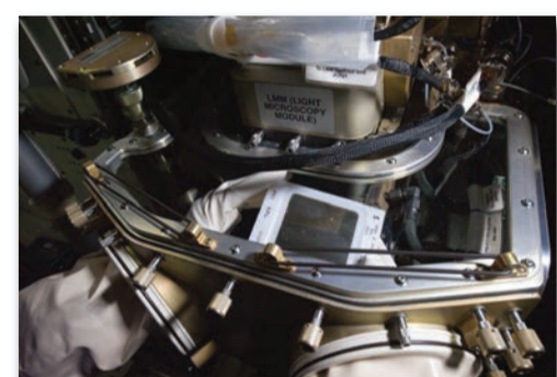
OptiCells™ being loaded into LMM.
