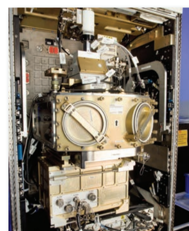
LMM mounted in the FIR rack.
