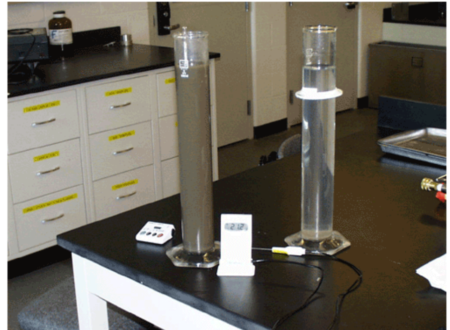
Figure 5-6. Soil hydrometer apparatus ( http://www.ce.siu.edu/ ).
