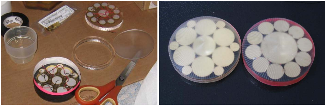
Fig. 3. (Color online) Multi-ceramic sensor fabrication – total sensor area equal to 65 cm 2 . Left: intermediate stage of fabrication showing ceramic and wiring in mold before adding epoxy. Right: Complete units before final mounting.
