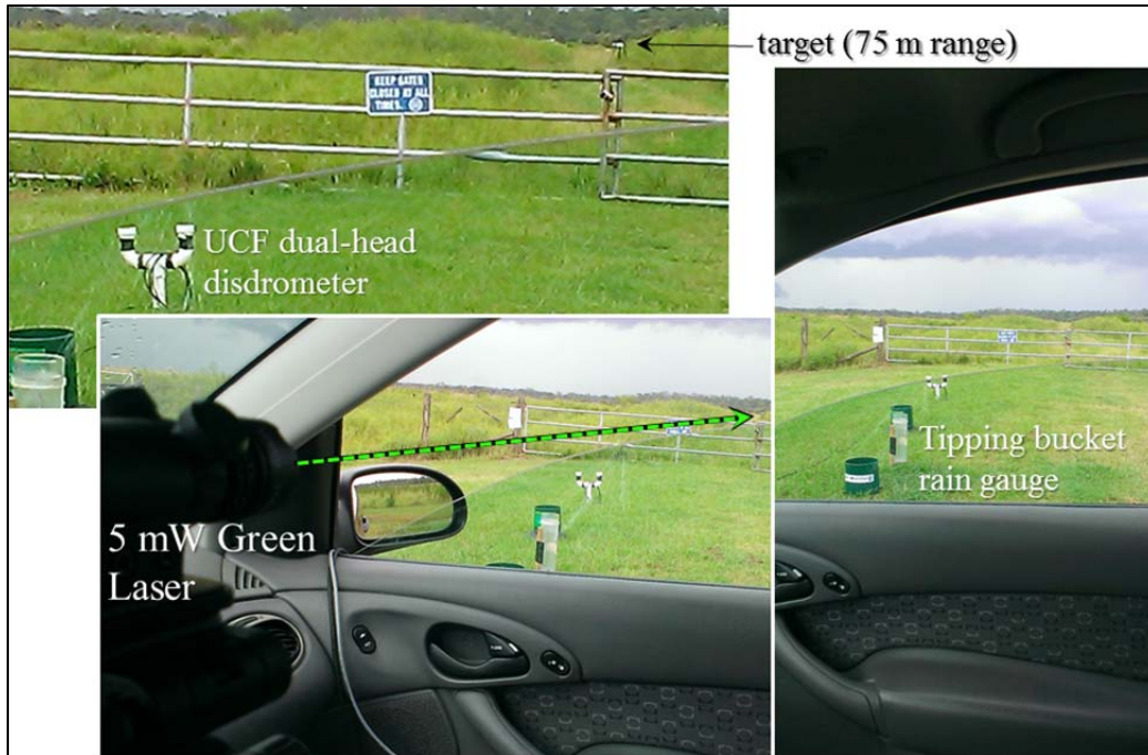
Fig. 7. Equipment setup: Top left: tipping bucket, accumulation gauge and laser target barely visible in background; Bottom left: laser and camera set up with all electronics inside of a vehicle, powered by car battery; Right: tipping buckets, rain gauge, and UCF-DHD shown through vehicle window.
