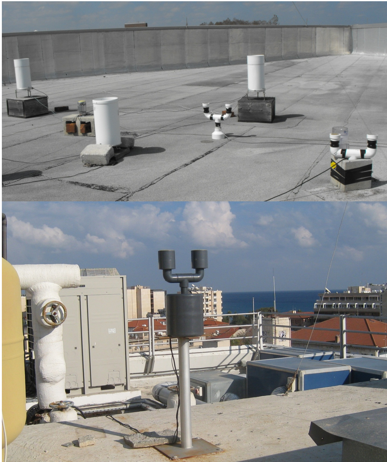
Fig. 1. (Color online) Top: Roof of UCF Engineering Building, showing three tipping bucket rain gauges (white cylinders) and three disdrometers: Joss disdrometer on left, and two UCF-DHD disdrometers in center and far right. Bottom: CUT-DHD on the roof of the Cyprus University of Technology.
