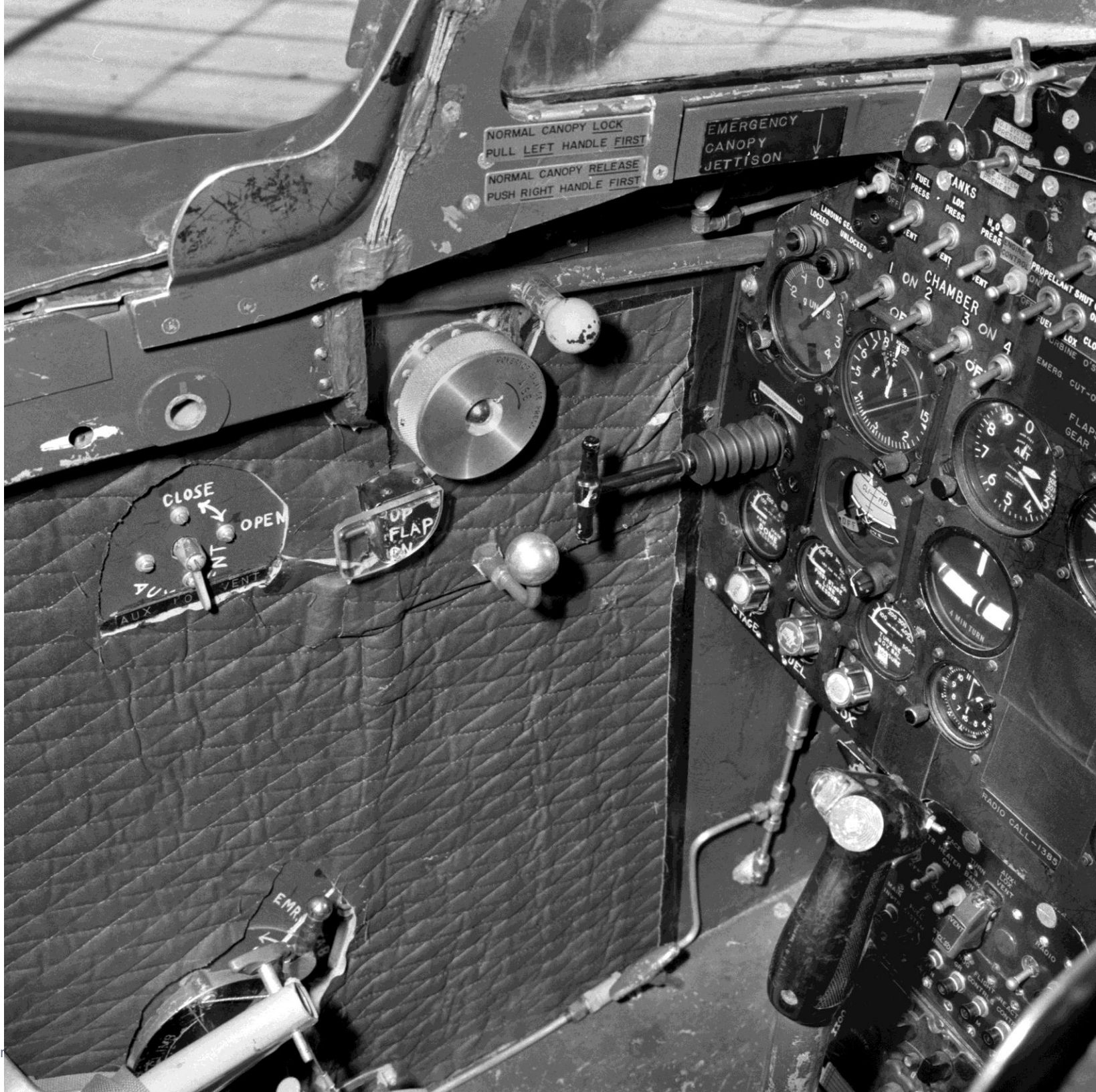
The RCS controller in the X-1B sticking out from the left side of the instrument panel.
