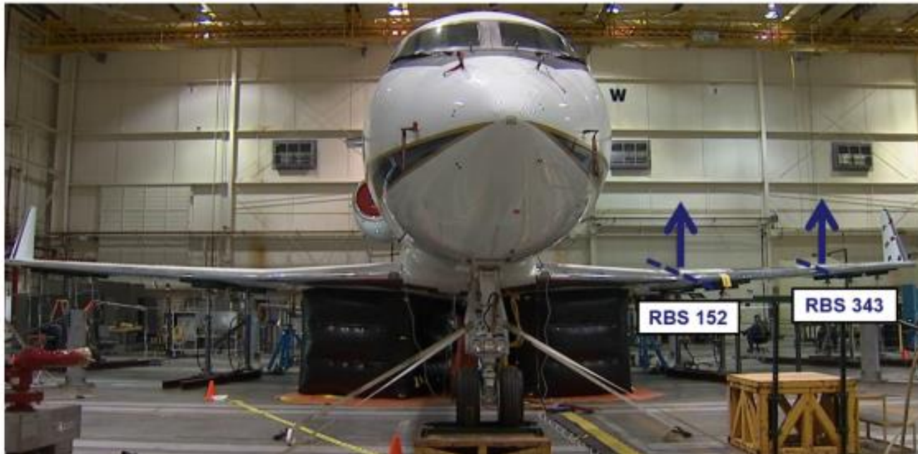
Photograph of hydraulic up load case with aircraft supported on airbag
