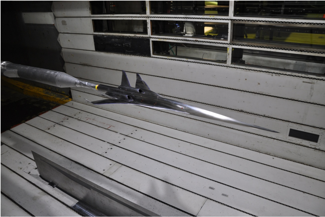
Figure 4-9. PM Model Installed in the NASA ARC 11-Foot Wind Tunnel.
