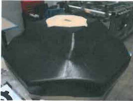
Figure 9: Top half of structure on foam tool
