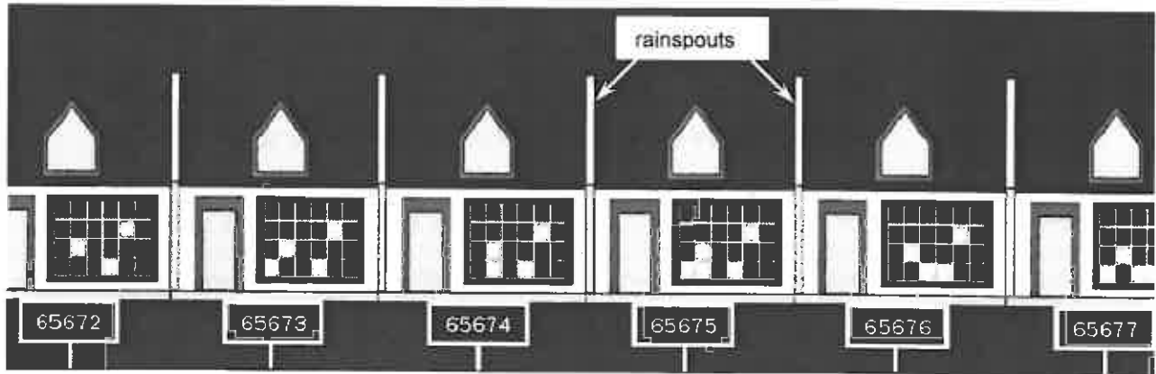
Figure 5 – digital photo of several adjacent townhouses. An image process recognizes the address of each house by its lamps and measures the apparent position of the rainspouts with respect to the camera's pixel columns with extremely high finesse
