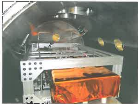
Figure 7. LTCS Demonstration Unit Thermal Mass Installed in Thermal Vacuum Chamber
