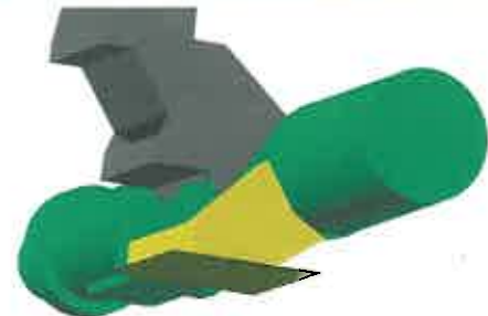
Figure 10. Damper Survival Heater Bracket The late addition of the aluminum bracket (yellow in model picture) created a high conductivity parallel path to the low conductivity hinge bracket
