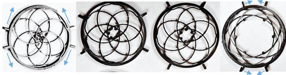
Figure 2. Example of a compliant iris mechanism.
