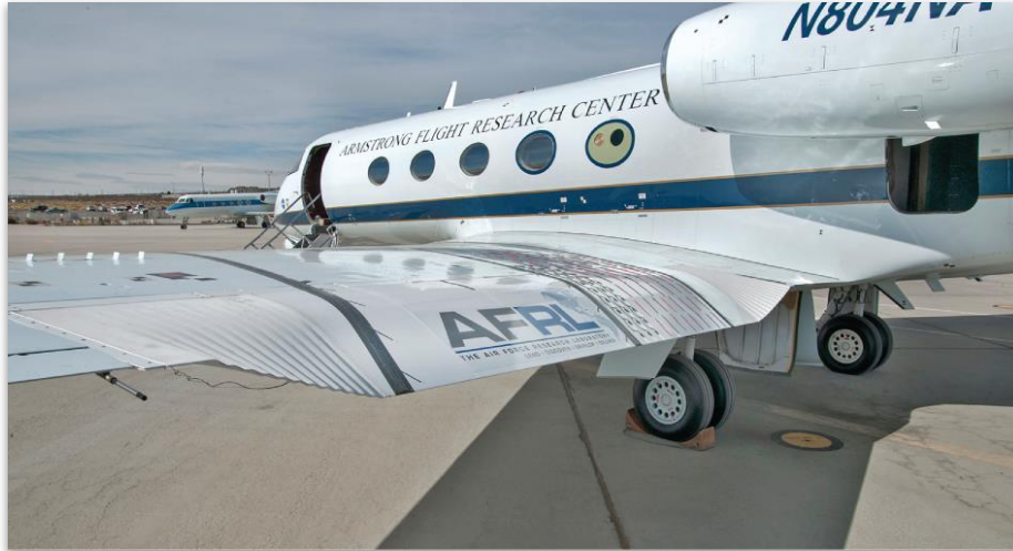
Figure 1. The Adaptive Compliant Trailing Edge flaps installed on the Gulfstream III Subsonic Research Aircraft Testbed at a flap deflection of 20°.
