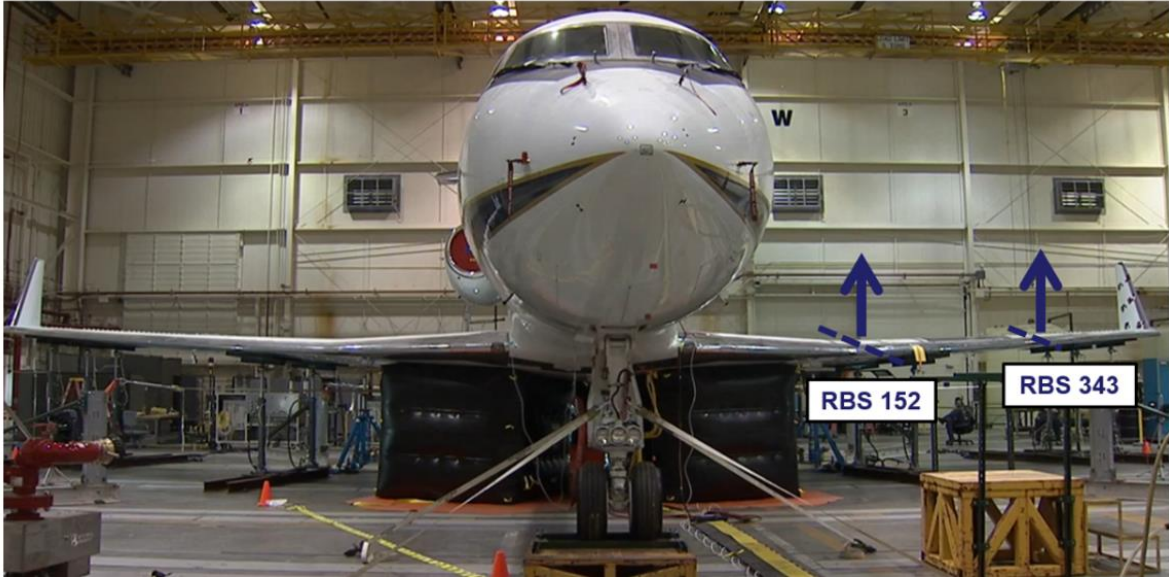
Figure 7. Photograph of hydraulic up load case with aircraft supported on airbag.
