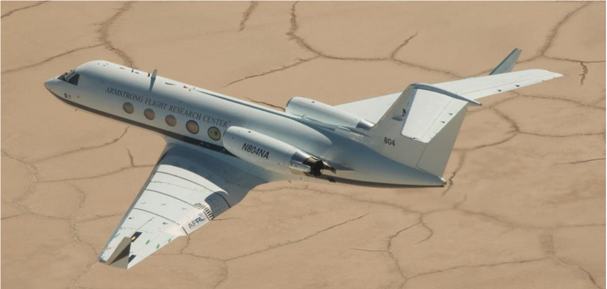
Figure 1. Modified Gulfstream III is the test bed aircraft used for ACTE flexible-flap research.
