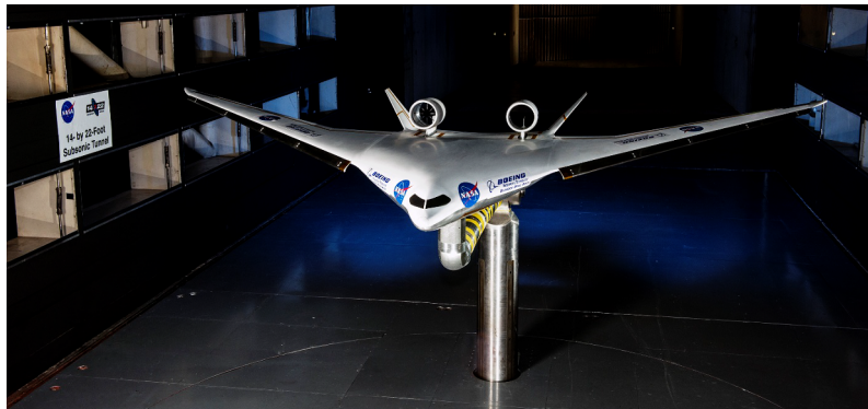
Figure 3. HWB model cruise configuration in NASA LaRC 14’x22’ wind tunnel.
