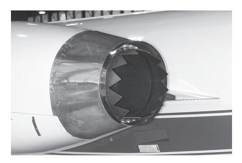
This early design of chevron nozzles—with the sawtooth edges—was installed on a NASA Learjet in 2001 to test how far the chevron edges could penetrate the airflow to reduce the most noise without reducing engine thrust beyond an acceptable level. A later design of the nozzles, which reduced engine noise up to three decibels, has since been included on engines for the Boeing 747-8 and 787 aircraft. Image credit: NASA
