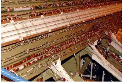
A damaged wire found during wiring inspections in Columbia's payload bay following STS-93, caused a short circuit in two separate main engine controllers on launch.
