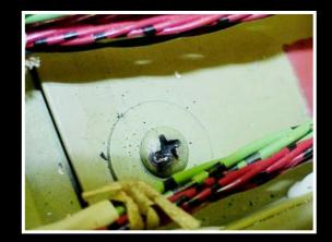
Wiring in the mid-body payload bay normally covered; records indicate covers last removed during Orbiter Maintenance Down Period (OMDP) 4 years earlier in the Palmdale depot facility.
