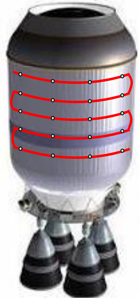
Example hyFOSS fiber layout
