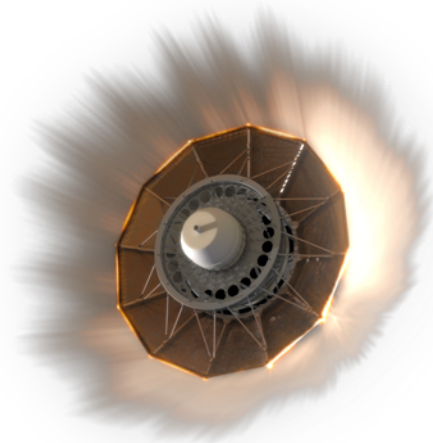
6 m diameter ADEPT-Venus in cruise (left) and entry (right) configurations
