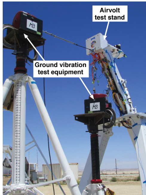
Figure 18. Test stand ground vibration testing.
