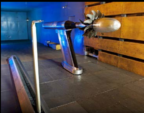
Open rotor installed in NASA wind tunnel (2010)
