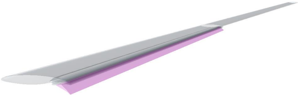
Figure-3.1.3(a): The D8.5 wing with flap in different positions during deployment
