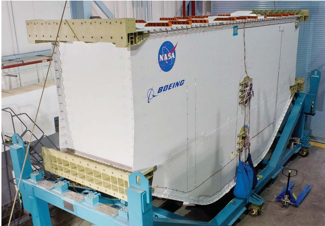
Figure 1: photograph of the large-scale multi-bay fuselage test article in a holding fixture
