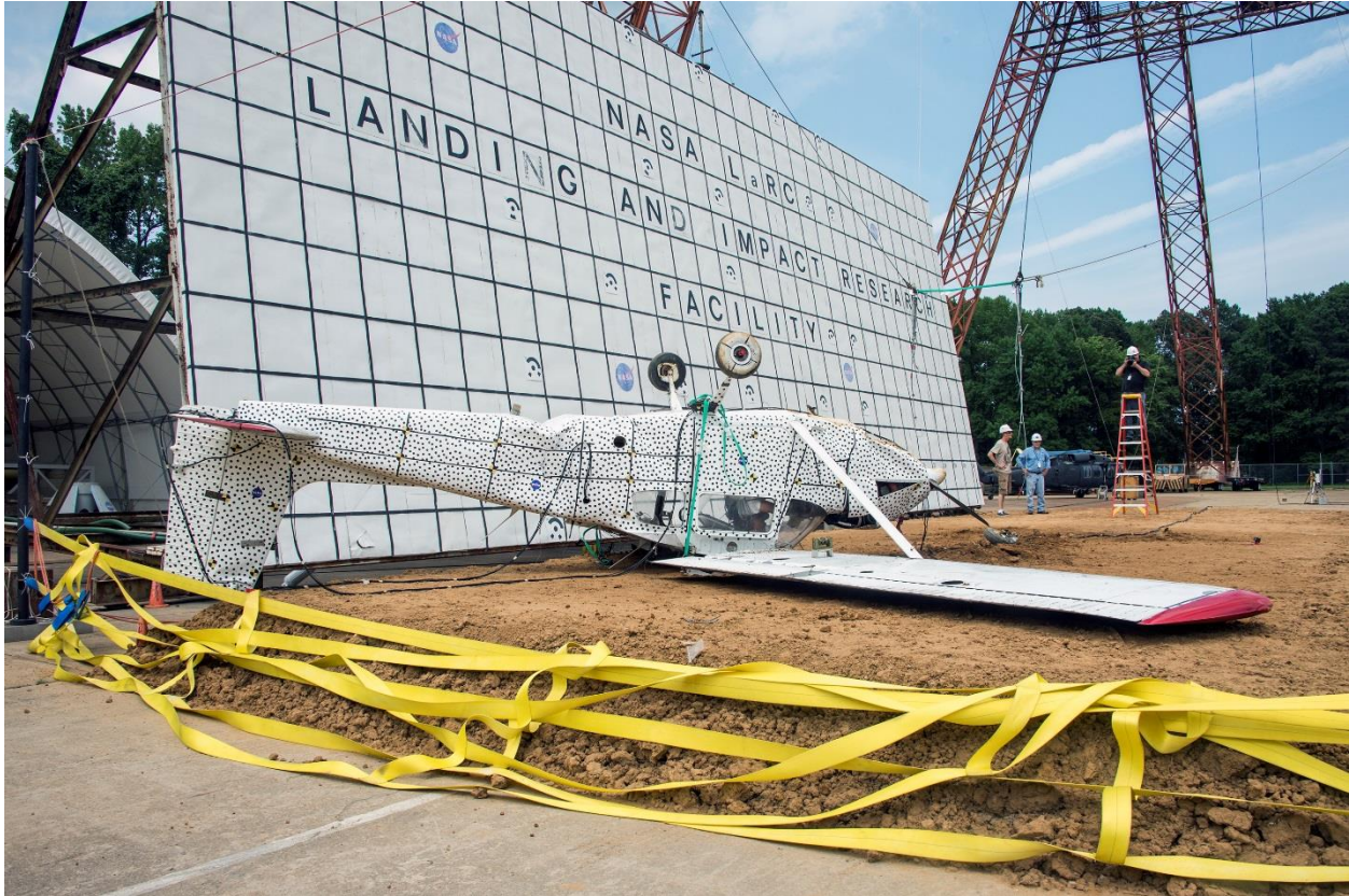
Figure 25 – Test 2 – Post-test pilot side tail damage
