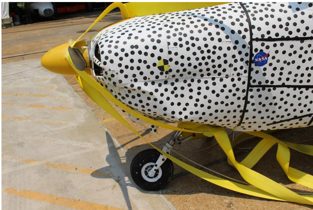
Figure 13 - Test 1 – Post-test nose buckling and landing gear orientation
