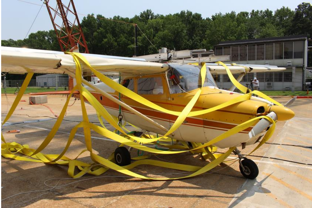
Figure 14 - Test 1 – Post-test wing damage
