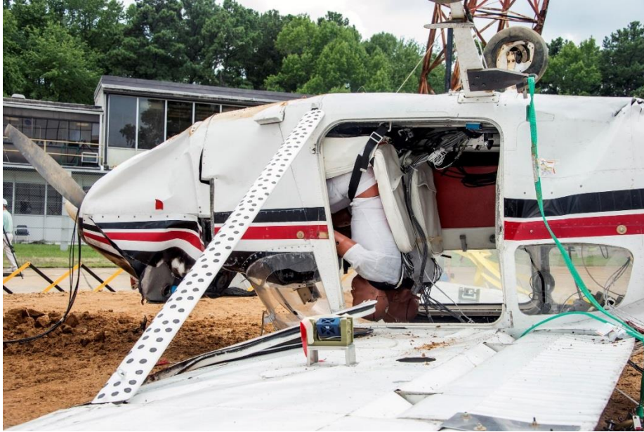
Figure 23 – Test 2 – Post-test airframe damage - Nose and co-pilot side cabin
