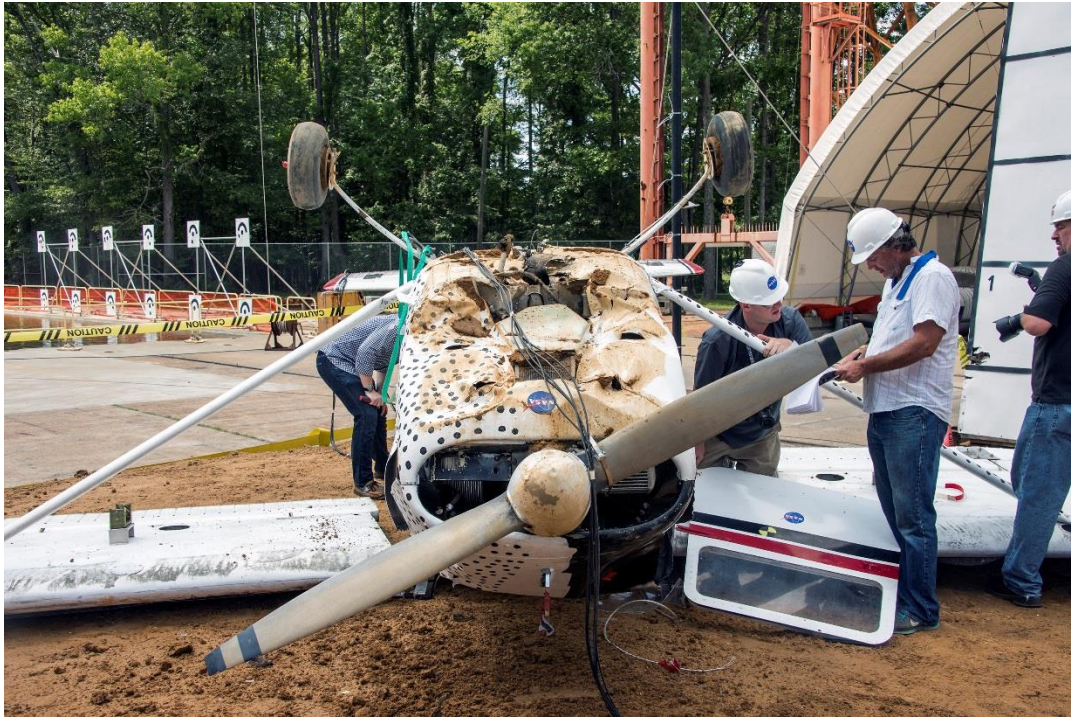
Figure 22 – Test 2 – Post-test nose damage
