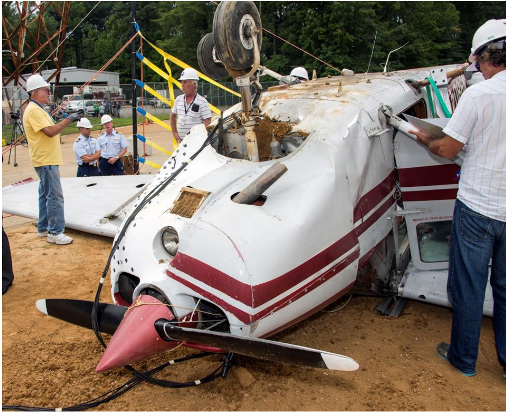
Figure 33 – Test 3 – Post-test nose damage
