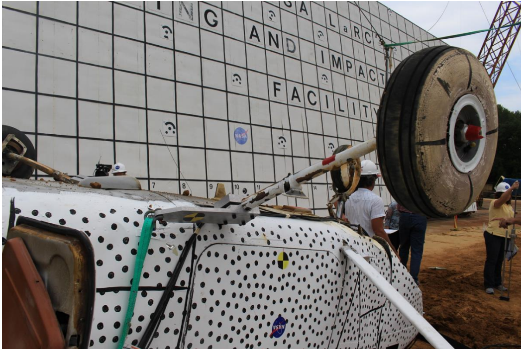
Figure 34 – Test 3 – Post-test landing gear deformation
