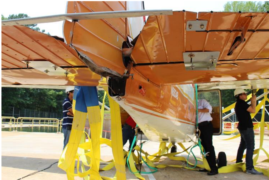
Figure 15 - Test 1 – Post-test tail damage
