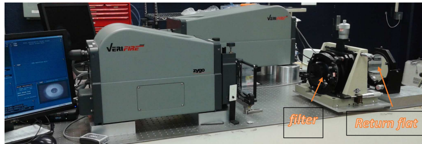
Figure 3. Transmitted wavefront error measurements setup showing an infrared interferometer (1,550 nm) and filter sample in a double pass configuration. A fold flat mirror is shown on the right side of the image behind the test filter mount.
