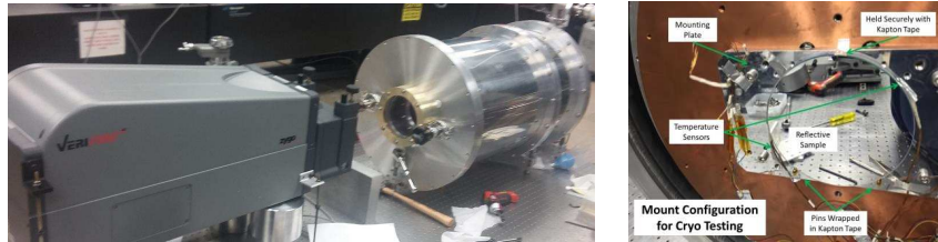
Figure 2. Left: The setup showing interferometer (left) and cryostat (right) for performing interferometric measurements at cryogenic temperatures. Right: Filter mounting scheme inside cryostat shown on left image.
