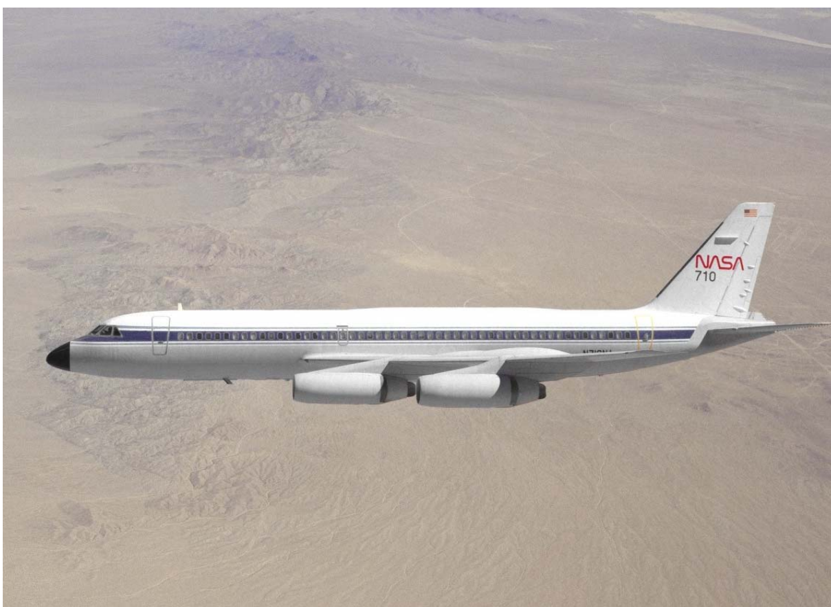
Figure 1. National Aeronautics and Space Administration (NASA) Ames Airborne Laboratory, the prototype CV-990 commercial aircraft acquired by NASA and converted by NASA Ames Research Center to the Airborne Science Laboratory, a platform for radar and optical experiments.
