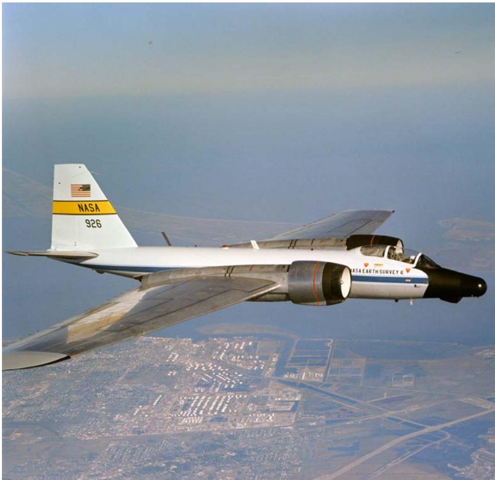
Figure 10. Johnson Space Center Earth Resources WB-57 Canberra aircraft used for the JSC X-band data acquisitions.
