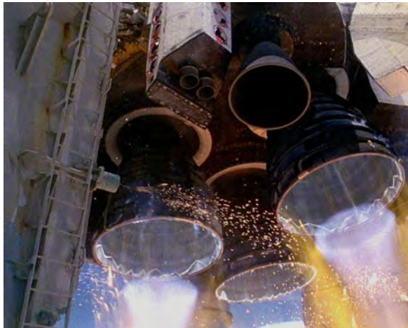
Figure 1: Image of three full-scale liquid propellant engines undergoing staggered startup (Courtesy: NASA).
