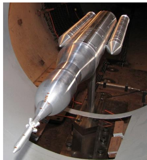
Figure 1 SLS Hot-Fire model installed in the LENS II facility.
