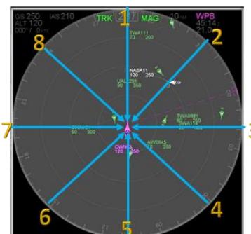
Figure 1: CSD depicting ownship at center, with 8 intruder approach geometries and background traffic
