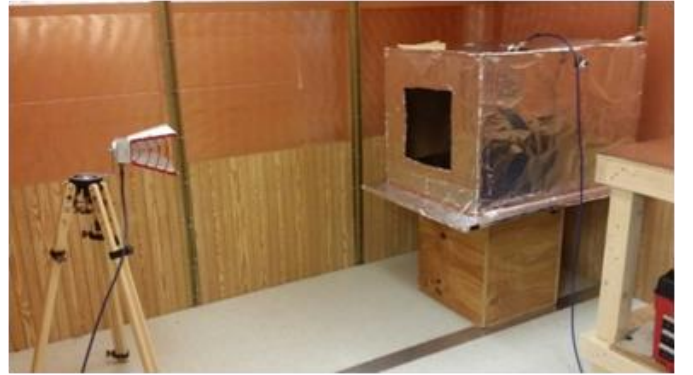
Figure 3 Canonical problem test configuration in NASA KSC reverberation chamber.
