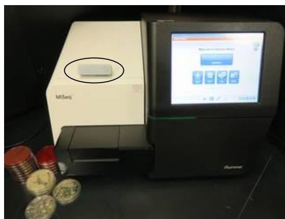
Figure 2. The MinION™ device (circled) sits atop the Illumina MiSeq sequencer. The MinION™ device is a nanopore sequencer that weighs less than 150 g, and occupies a volume of less than 100 cm 3 .
