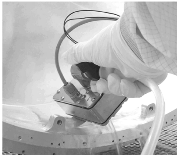
Fig. 4-10. A stream of megasonically energized UPW generated by a portable wand is used to clean the canister base.
