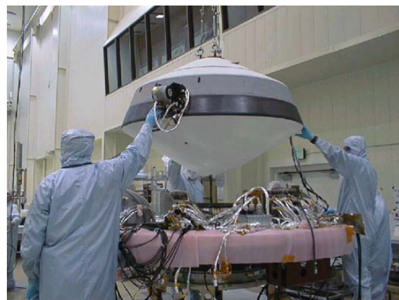
Fig. 5-3. The sample return capsule for Genesis was assembled and tested within several multi-story spacecraft assembly rooms at Lockheed Martin Astronautics in Denver, Colorado.
