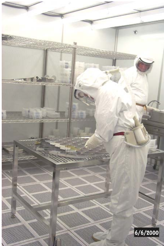
Fig. 5-4. Dryden suit completely envelops person. Self-contained battery motor forces exhaled breath through HEPA filters.
