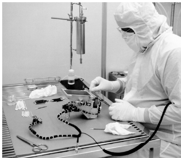
Fig 4-8. Electronics Box cleaning with IPA-dampened swabs.
