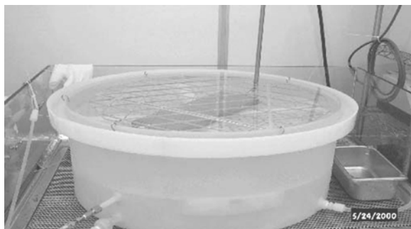
Fig. 4-4. Cascade both flow of UPW is 2 gallons/min. An array frame is being cleaned in this view. Below the array frame, the rectangular ultrasonic generator is visible.
