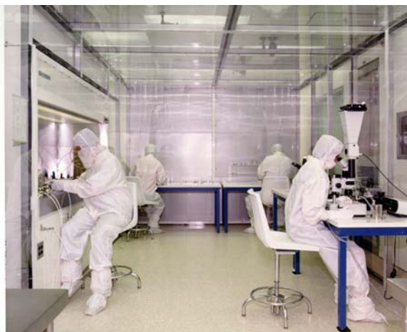
Fig. 5-1. Class 100 laminar flow tunnel for preparing and examining interplanetary dust particles captured in the stratosphere
