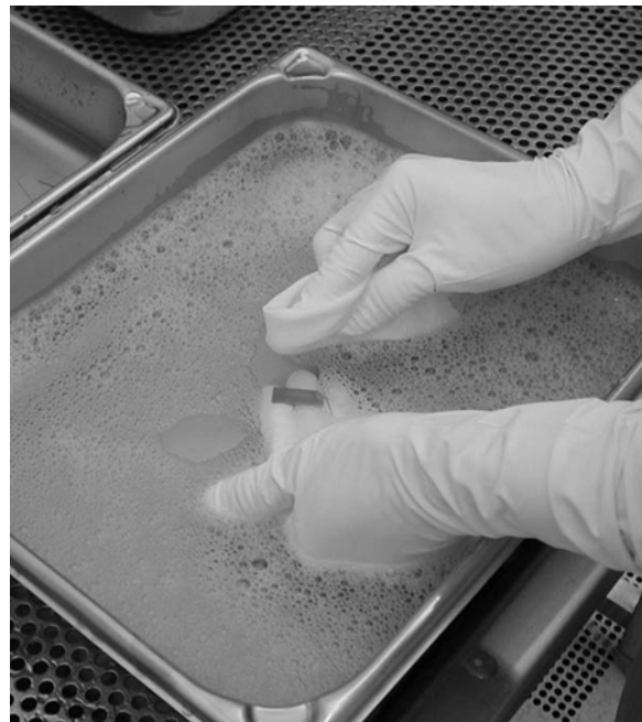
Fig. 4-3. Precleaning by scrubbing in surfactant solution. Item remained submerged until rinsing to preclude drying of detergent on surface.
