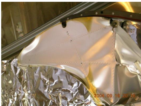
Fig. 6. Close-up of canister thermal shield illustrating shading from direct solar radiation (see fig. 3).
