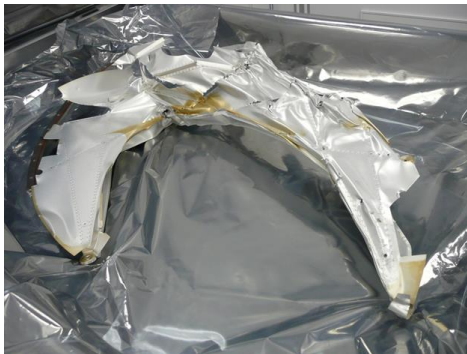
Fig. 5. Canister thermal shield as returned after hard landing. Brown areas are where solar radiation darkened a molecular film.
