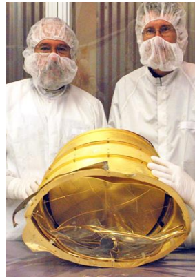
Fig. 8. Concentrator as recovered in Utah. Interior portions of the structure experienced operational effects of focusing voltage. [18]
