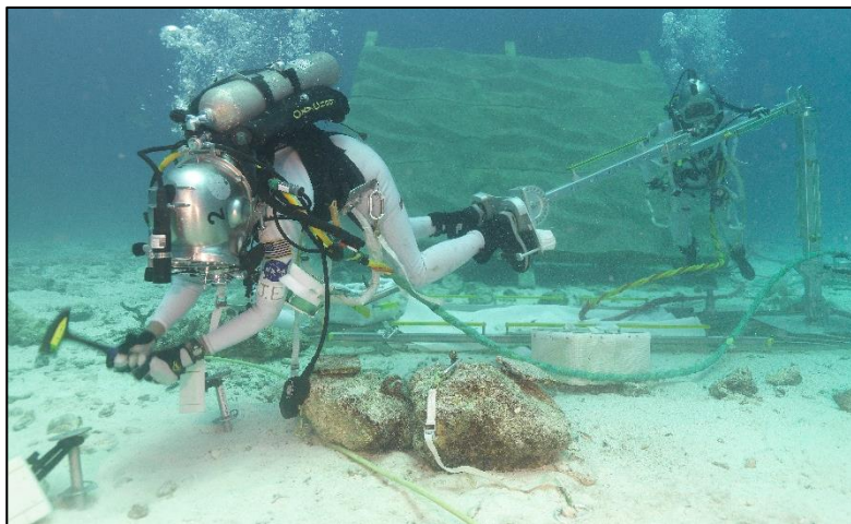
Figure 2. Science Package Deployment, Body Stabilized with a Foot Restraint on a Boom during the NEEMO 18 mission.
