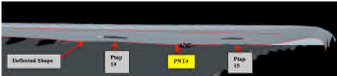
Figure 22. Cross section of 90° gore: 20 lbf/in measured tension, 100 psf and 0° AoA.
