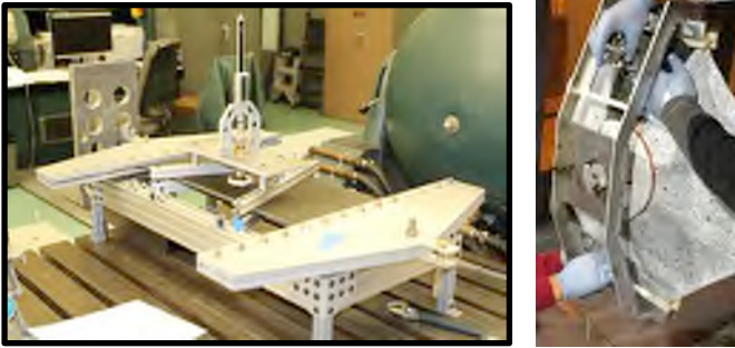
Figure 5. Calibration rig (left) and deflection measurement tool (right).
