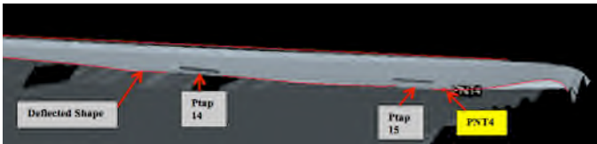
Figure 23. Cross section of 90° gore: 5 lbf/in nut setting, 100 psf and 0° AoA.
