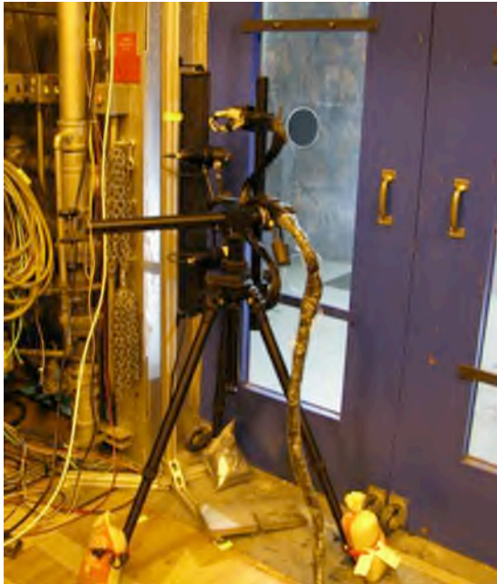
Figure 8. Photogrammetry cameras mounted sideways on a tripod outside the 7x10 tunnel.
