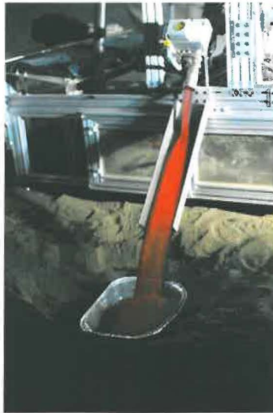
Figure 8. Hot tephra at \sim 1000 C flowing out of Gemco, Inc valve attached to the bottom of the ROxygen I reactor shown in Fig. 7.
