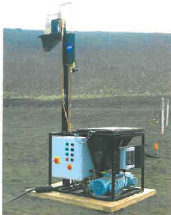
Figure 2. Automated closed-loop pneumatic regolith feed system developed for the Carbothermal reactor ISRU field test at Mauna Kea in 2010.
