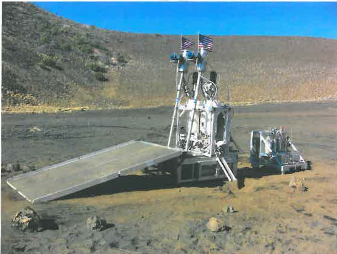
Figure 7. The ROxygen I oxygen production system at the 2008 ISRU field test site in Wahine Valley on Mauna Kea, Hawai'i. The inclined auger regolith transfer system is shown projecting upwards at the top of the ramp to feed Tephra into the reactor.
