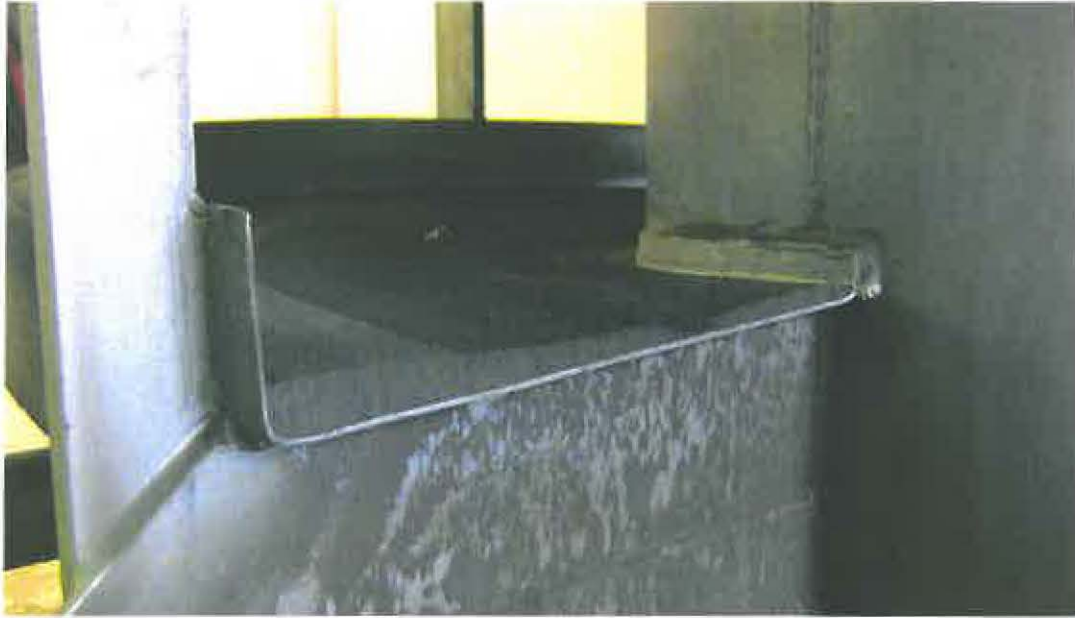
Figure 10. Layer of JSC-1A on spiral elevator test fixture (Carman Industries, Inc.)
