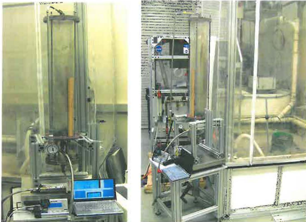
Figure 3. Experimental setup to determine the mass flow rate of JSC-1A using dry compressed air both as the convey gas and to fluidize the lunar regolith simulant contained in the acrylic supply cylinder show in the front view (left image) and side view (right image). The right image shows how granular material is educted at the bottom of the supply cylinder and flows freely along a horizontal pipe into an open bucket located inside an enclosure that keeps air borne particulates inside.
