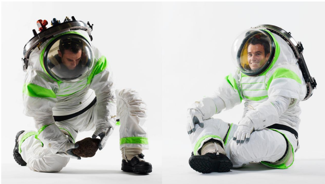
Figure 1. Z-1 Planetary Space Suit Prototype
