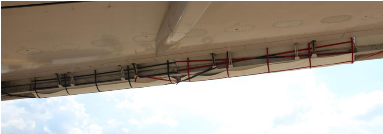
Figure 53: Slat Covers Installed From Lower Surface
