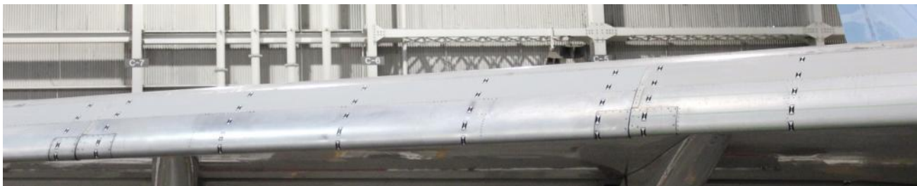
Figure 32: Painted Lines and Photo Targets on Slats (no IAM panels installed)
