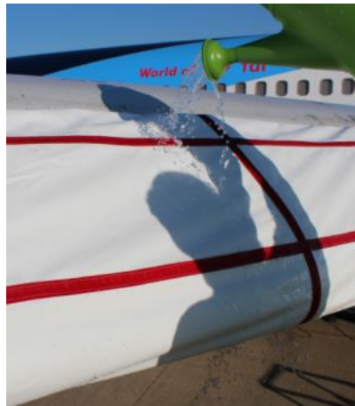
Figure 54: Testing for Water Proofing
