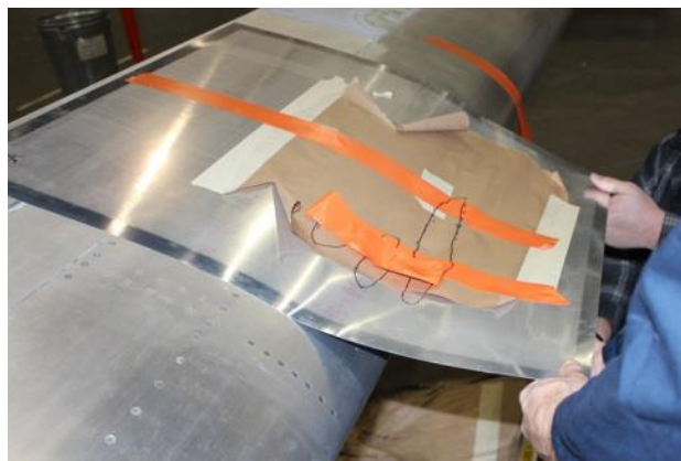
Figure 40: Peel IAM Panel Away From Slat (Upper Surface View)
