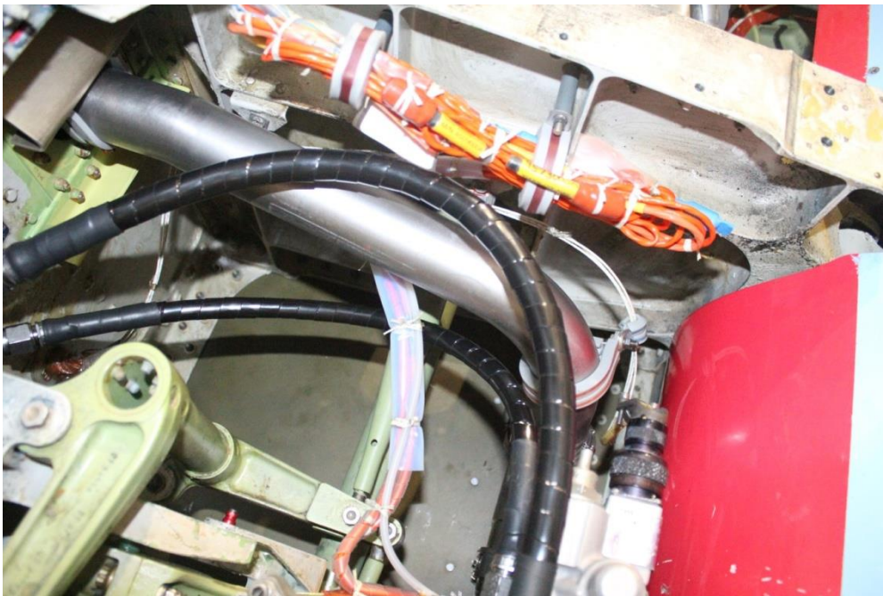
Figure 9: Hydraulic lines and AFC ducting
