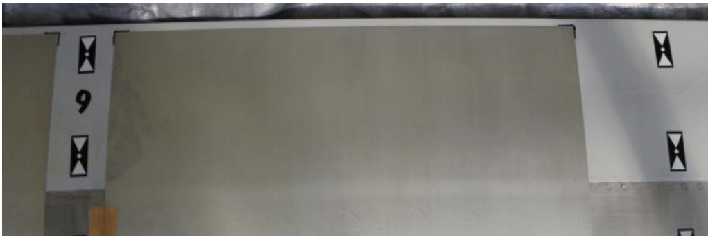
Figure 36: Panel Installed With Upper Trailing Edge Corner Locating Marks
