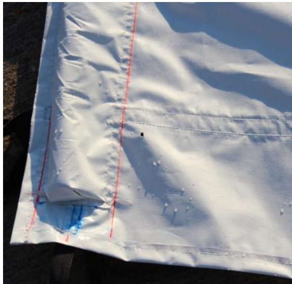
Figure 55: Drain Path for Water Pooling at Covers Lowest Point
