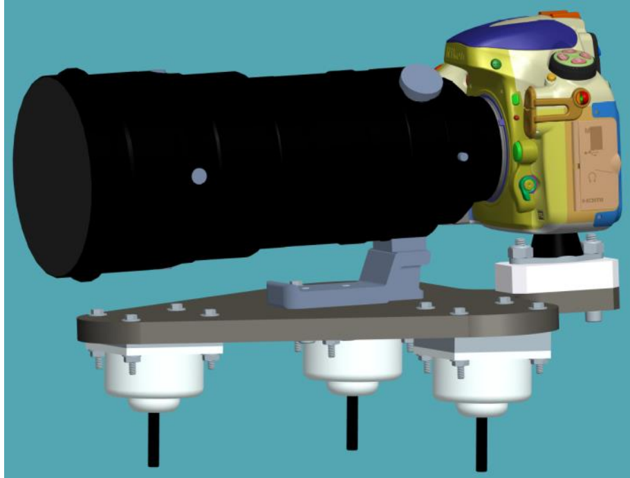
Figure 24: NASA Mount Design with Camera Attached
