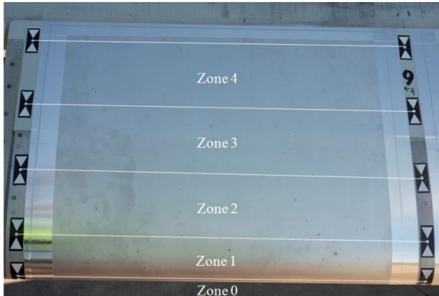
Figure 57: Panel Zone Numbering (View from Above)
