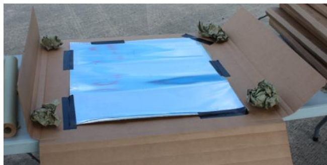
Figure 41: Flat Removed IAM Panel with Edge Marked for Area Lines
