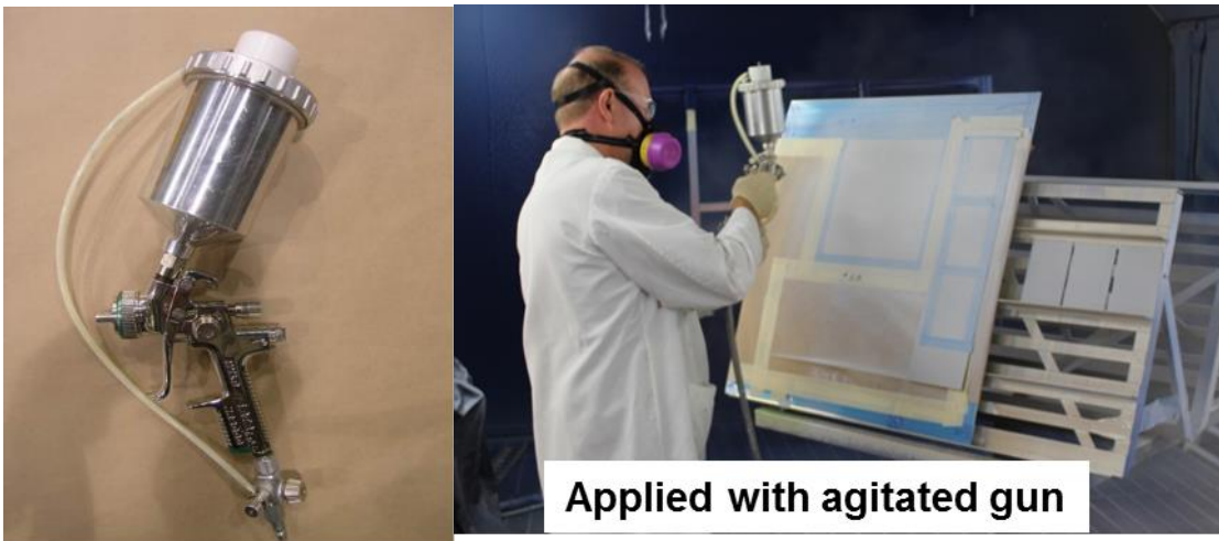
Figure 47: Sata NR2000 D=Gravity Fed Paint Gun with Agitator
