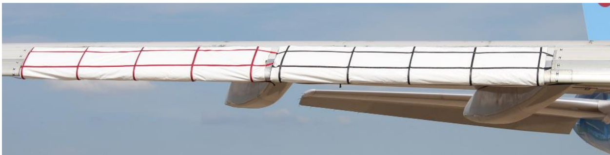
Figure 52: Slat Covers Installed
