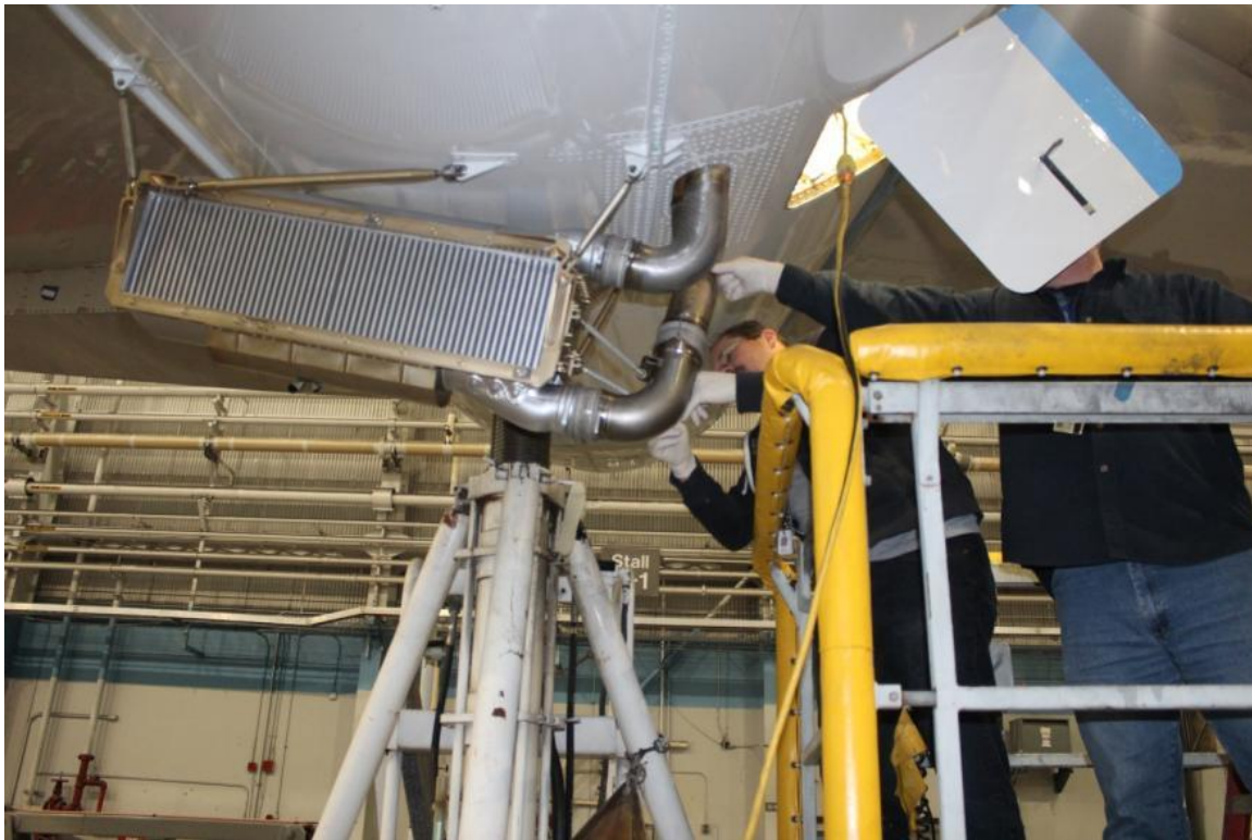
Figure 10: Installation of the heat exchanger below the aft fuselage
