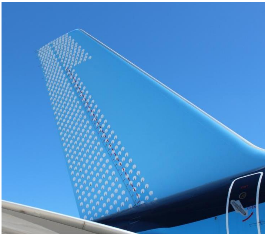
Figure 12: Flow cone installation on the vertical fin and rudder
