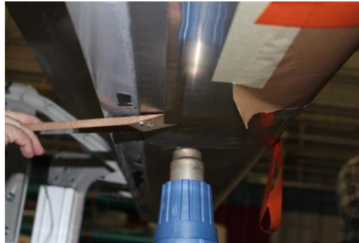
Figure 39: Peel substrate away from slat surface (Lower Surface View)
