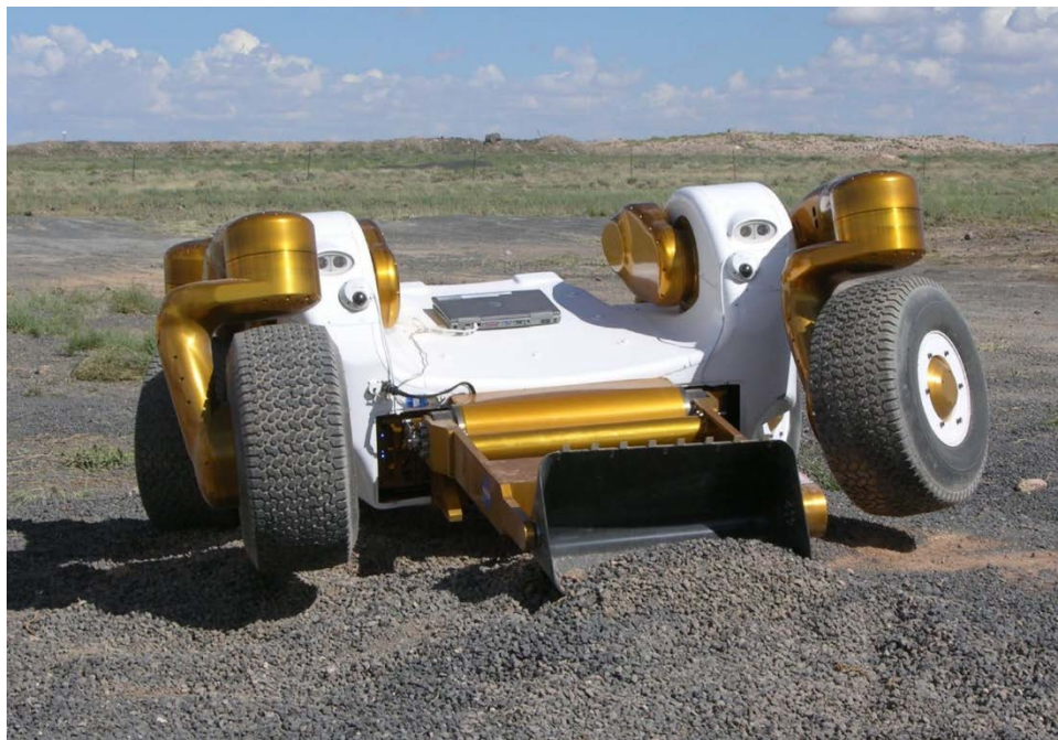
Figure 10.—The Digger shoulder actuation is strong enough to lift the front wheels of Centaur 2 off the ground.
