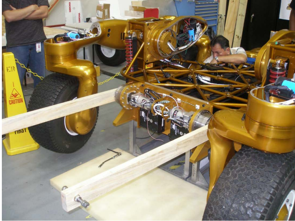
Figure 8.—At JSC, C2 with Digger Base Plate mounted, and temporary arms for shoulder actuation coordination testing.
