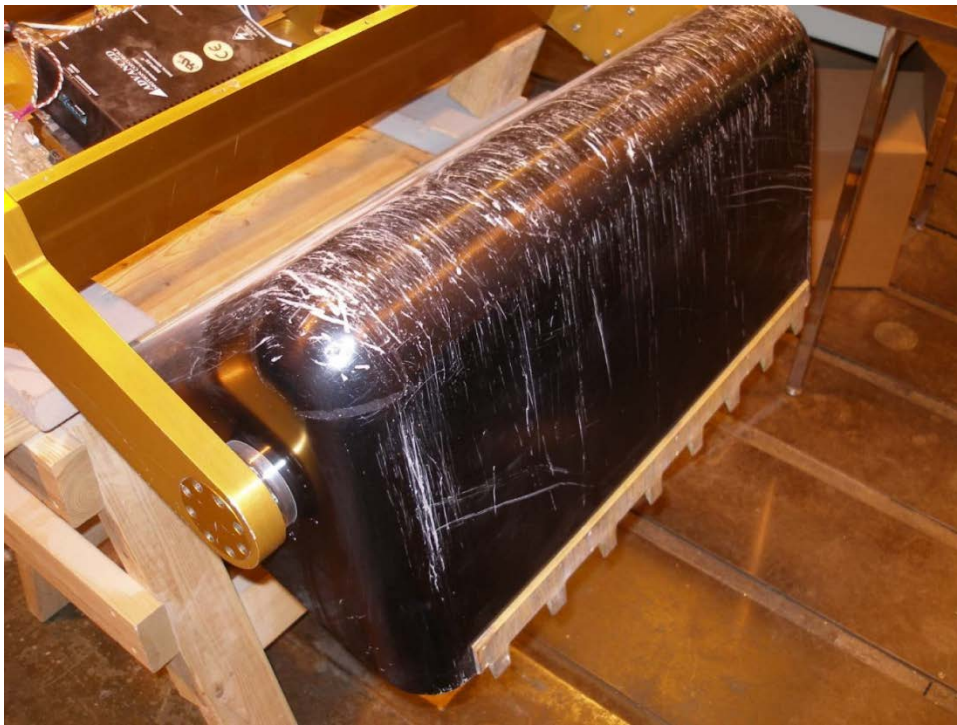
Figure 11.—During Desert Rats 2010, the black oxide coating of the aluminum bucket got scratched and gouged.
