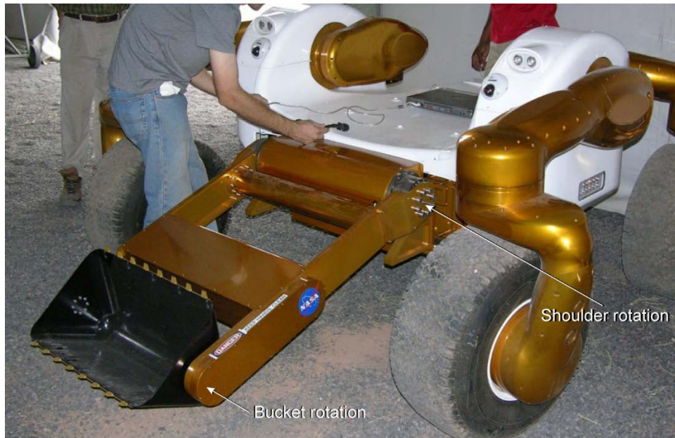
Figure 2.—Early at Desert RATS 2010, Centaur 2 with GRC Digger mounted, preparing to test.
