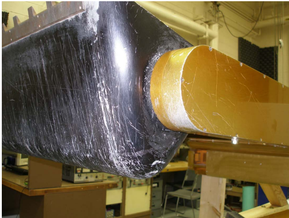
Figure 18.—After Desert Rats 2011, the black paint coating of the bucket is scratched, as is the chain guard.
