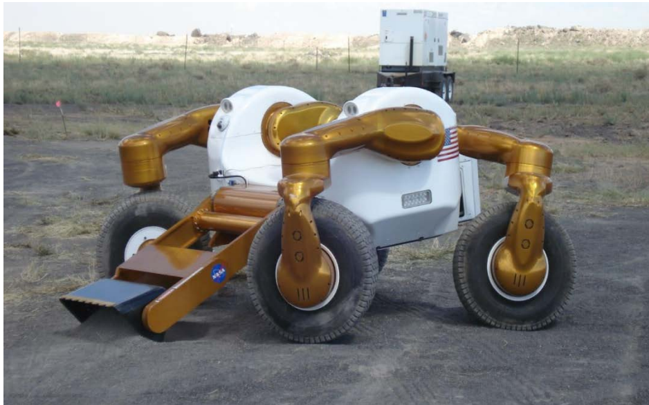
Figure 16.—Because each wheel can be independently steered, Centaur 2 can twist and crab, potentially putting great side loads on the Digger.
