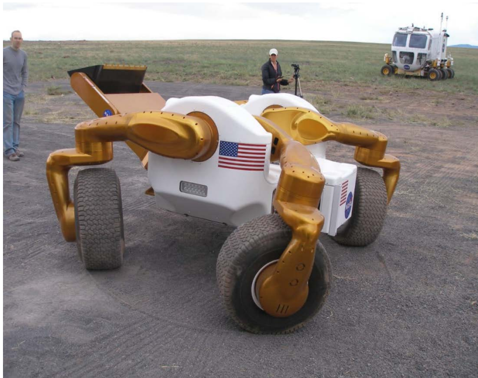
Figure 20.—Centaur 2 can turn on its own footprint.
