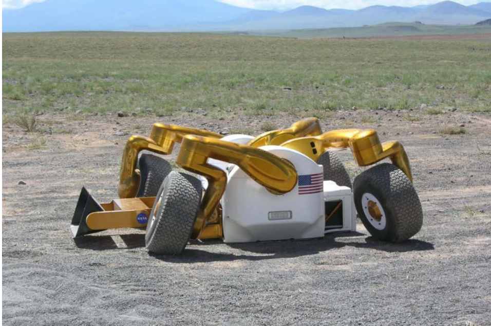
Figure 21.—Using its articulated bogies, Centaur 2 can lower its chassis to the ground, even with the wheels turned for crab-travel.
