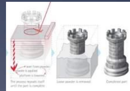
Additive manufacturing with laser sintering (3D printer principle)
