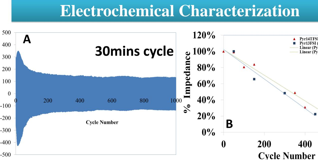
A. Voltage vs. Cycle Number of 0.5m LiTFSI in Pyr14TFSI symmetric cycling at 1mA/cm2, 30 mins cycle. B. % Impedance vs. cycle number for 0.5m LiTFSI in Pyr14TFSI and 0.5m LiFSI in Pyr13FSI
