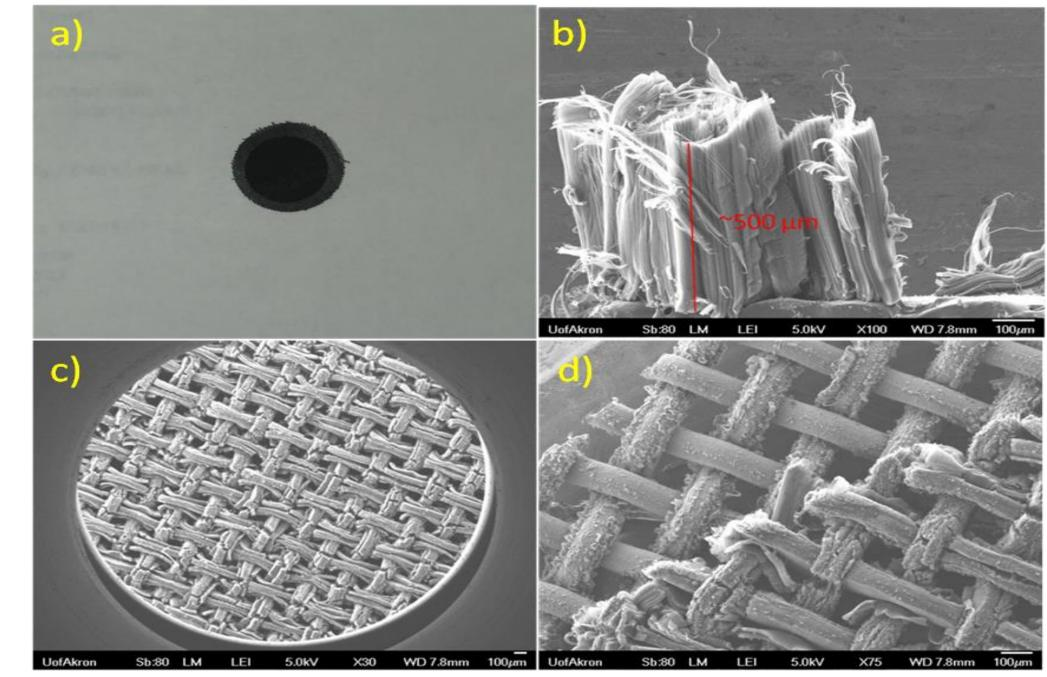
Vertically aligned carbon nanotubes (VACNT) directly grown on stainless steel mesh. The VACNT have a height of 500µm. U. of Akron
