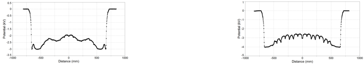
Fig.4. Differential potentials are shown for coupon #5: left panel- U_b= -3 kV; right panel- U_b= -4 kV.
