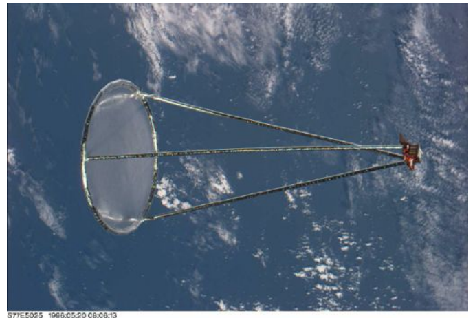
Fig. 6. Inflatable Antenna Experiment, a 14-meter diameter reflector demonstrated in orbit in 1996.
