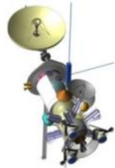
Neptune Systems Explorer ~3 kWe (9 Large RPS)
